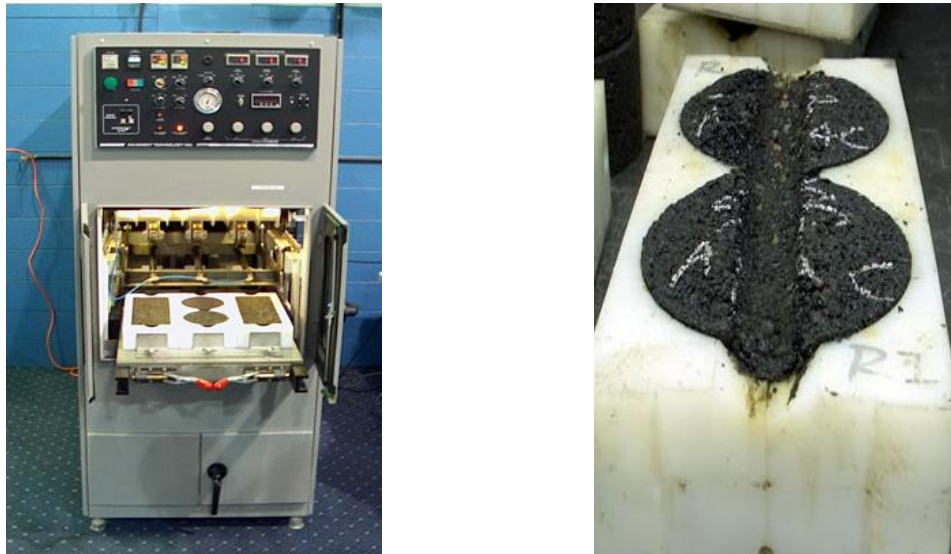
Figure 3.13 APA Test Station and Specimens after Testing
