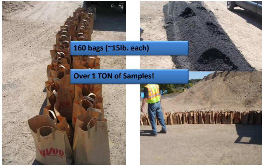
Figure 1.3 Field-mixed Loose Mixtures Delivered to the NDOR and UNL Laboratories
